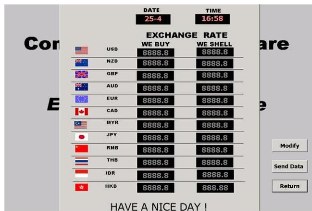
8) Firstly, click “Modify” then you can input the value to overwrite the previous data, then click the “Send Data” button, the PC will send the data you inputted to update the values shown on the Exchange Rate Indicating Board.
