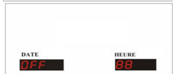
Press the "S" key again, the display will show as the right diagram, Then you can input your desired switch off minutes by pressing the numeric keys.
