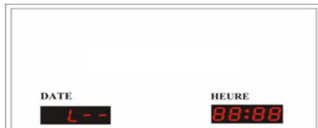
The “L- -“ indicates the brightness of the LED in the automatic adjusting mode, the board will adjust the brightness according to the environment light brightness.
