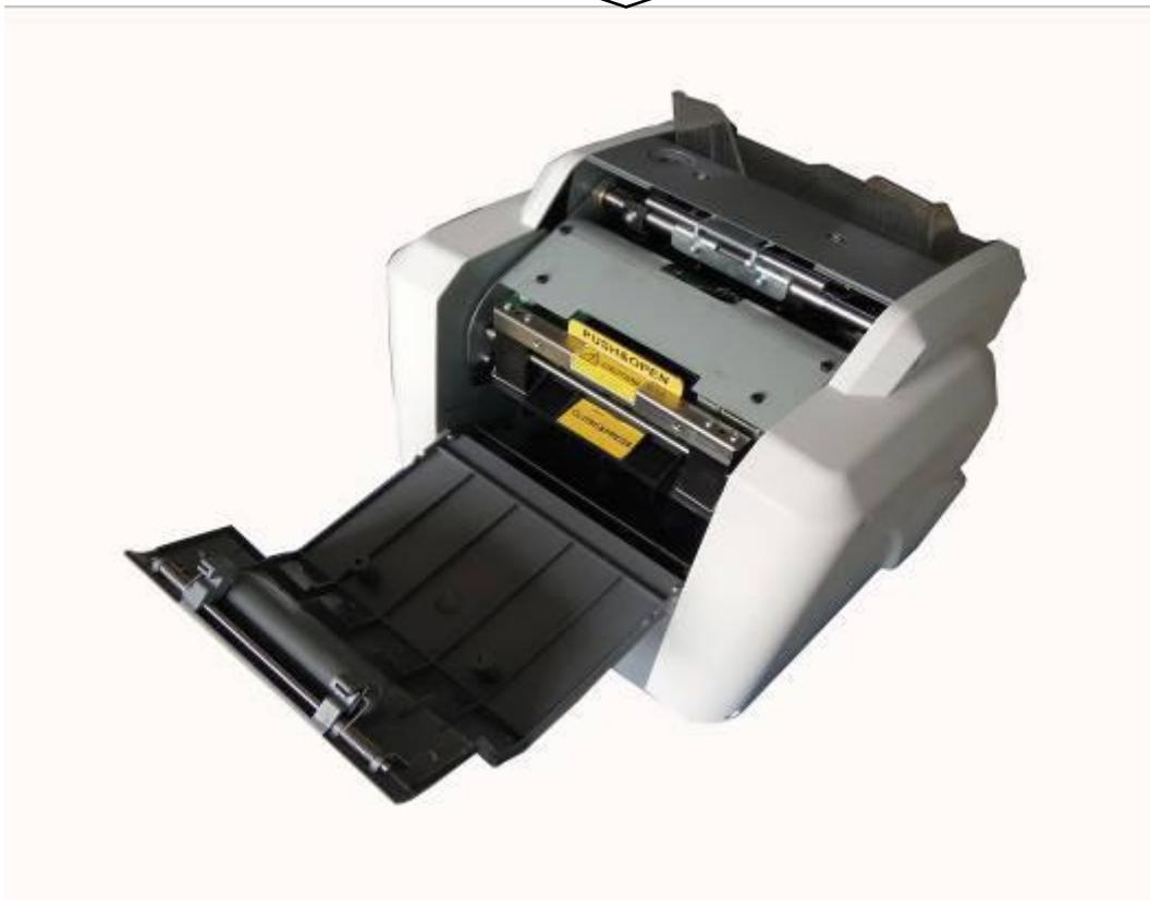
2) Press and push forward the metal bar to open the interior passage.
